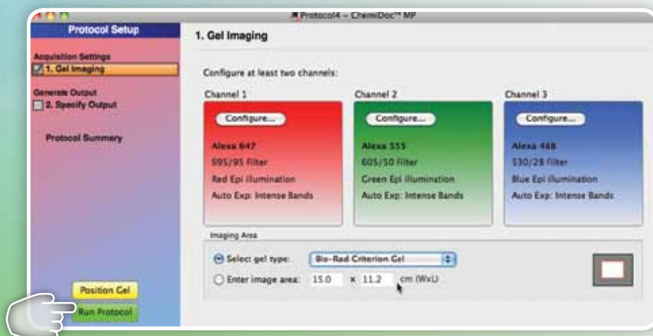
Fig. 9A. The application selected automatically determines the excitation sources and emission filters.
